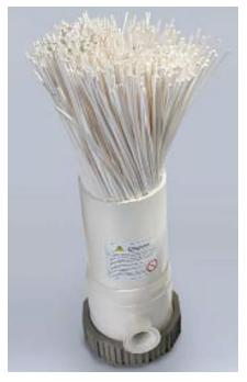
FIGURE 2A: This Pall Oenoflow membrane cartridge contains hollow fiber membrane tubes bundled together inside the cartridge. The lees travel down the inside of the tubes and the clarified material passes into the cartridge body and out of the system. The fiber diameter and length has been optimized for winery lees use.
