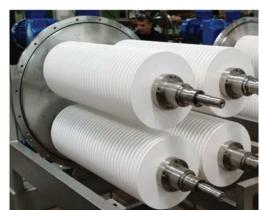
FIGURE 3B: Multiple ceramic discs are placed on horizontal shafts in Padovan's Dynamos lees filter, and each spindle rotates in the lees mixture.
