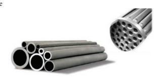
FIGURE 3D: The VLS system of sintered stainless steel membranes is similar to the Della Toffola system. However, these membranes are welded into the head as a unit. There are several different oxides that coat the inorganic material, with the two most common being titanium and zirconium. These metal oxides create the pore space for the membranes.
