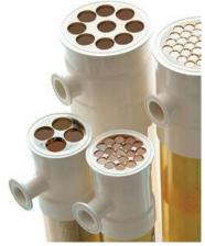
FIGURE 2B: This photo shows large bore hollow fiber membranes of different diameters in a Koch Separations lees filtration system. Koch wraps each membrane with reinforcing net to provide the structural support for the hollow fiber and to accommodate the viscosity of the process material so it can flow. In this photo, there are hollow fiber membranes of different diameters. Koch can select the appropriate diameter tube that optimizes the process characteristics for the customer's product.
