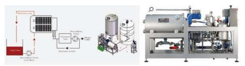
FIGURE 8: The Padovan Dynamos lees filter is similar to the Della Toffola system only in the material they use to construct their membranes. The company has created a novel crossflow dynamic system that works in viscous material. The flow path does not use a single path crossflow stream that returns to the primary feed tank. Instead they use a single path architecture using the spinning discs that eliminates the need to return retentate, and the tank is filtered in a single pass.
