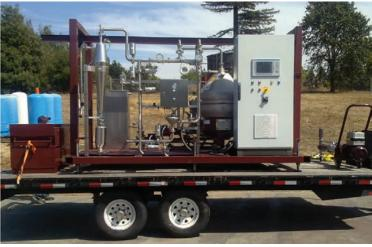
FIGURE 4: The Separator Technology Solutions STS 200 lees filtration system looks simple on the outside but is uniquely designed on the inside. The STS 200 can centrifuge heavy solid lees using their proprietary system and achieve good performance.
